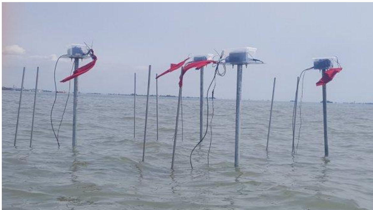
Repeatability test of the SOD rate measurement, with 4 benthic chambers placed in a small neighborhood.
